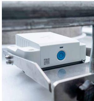
Micropilot FWR30 mounted on an IBC
